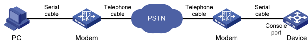
Figure 19 Set up a configuration terminal
